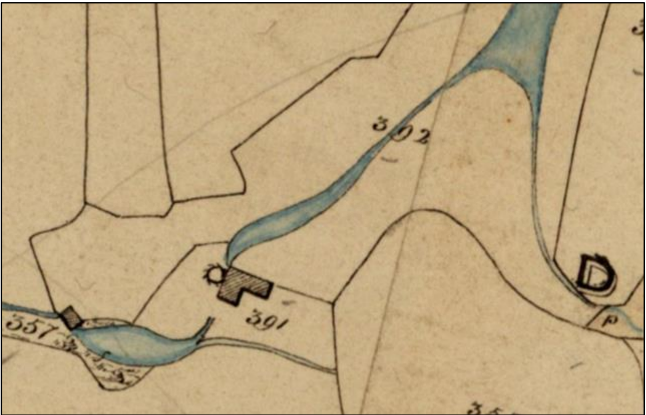
Figure 2. Extract from the Doultling Tithe Map of 1843. The Edge Tool Works is plot 391. The water-wheel at the upper buildings is shown rather diagrammatically, and the three mill ponds. (Map courtesy of Know Your Place - West of England)
